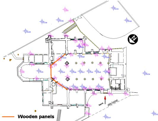
Figure 60: Overview of all the scan positions and the target configuration proposed by the authors
