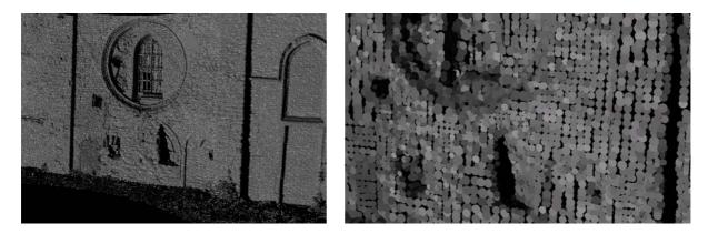
Figure 47: Result of laser splatting (left), close up of laser splatting (right)
