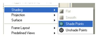
Figure 110: Shade the point cloud view for better understanding
