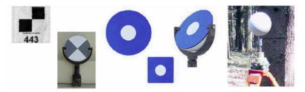
Figure 32: Artificial target types
