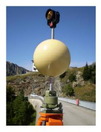
Figure 212: Painted wooden sphere with prism assembly, d=23.85cm
