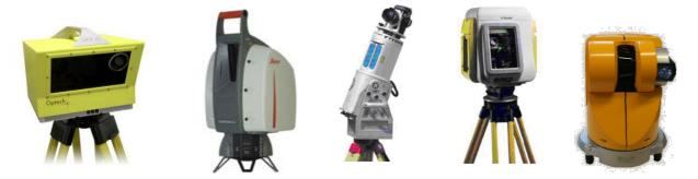
Figure 15: Commercially available Time-Of-Flight Laser Scanners
